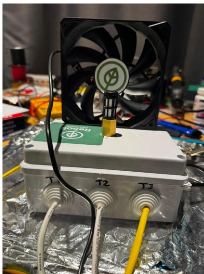
Photo taken by Resoil Network. Active fan system with temperature sensors integrated
